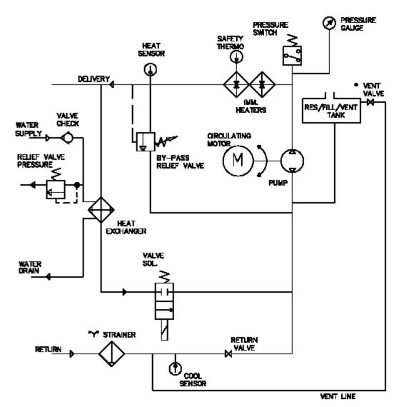
Note: The heat exchanger is optional, and the "Vent Valve" is also known as the "Blow-Off Valve."
